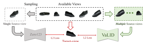
Figure 1. Compared to the previous method (Zero123 [18]), which can only receive a single image as input even when multiple images are available, the proposed architecture (VaLID) can accept variable input views in both training and inference. Thus it can learn a robust representation during training and can utilize more information in the inference time.
