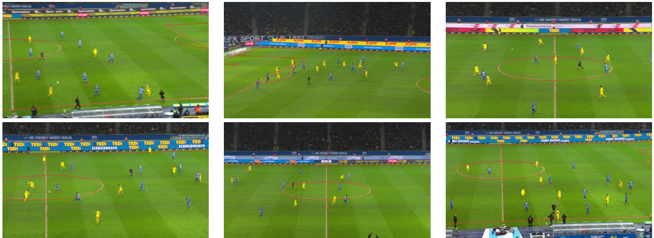
Figure 4. Qualitative evaluation of the 20 minutes sequence from the Bundesliga. One out of 10,000 images is displayed. Soccer field markings are reprojected in red using the estimated camera parameters \kappa .
