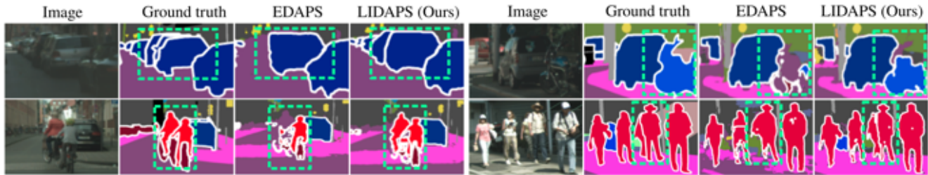
Figure 1. While previous SOTA methods for panoptic UDA such as EDAPS [52] achieve good semantic segmentation performance, they struggle to predict correct object boundaries and thus instance segmentation masks.
