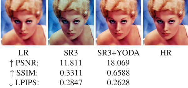
Figure 4. SR3 and SR3+YODA reconstructions, 64 → 256 (4×). SR3 suffers from color shifting, as also observed by [6, 36]. YODA solves this issue and produces higher-quality reconstructions.
