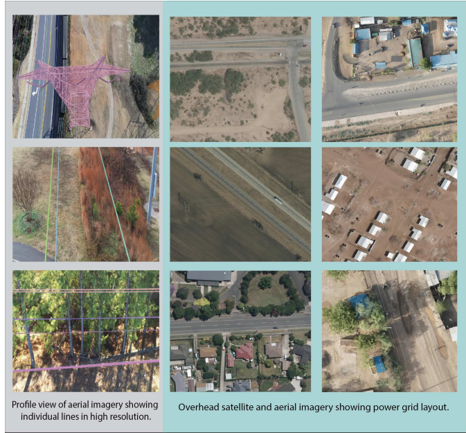
Figure 1. Profile views (left) better support mapping individual lines and tower structures, while overhead imagery (right) better supports mapping the layout of a power grid.
