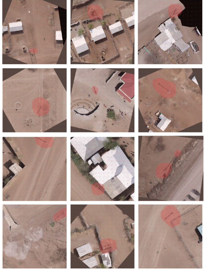
Figure 4. Test set sample images with predicted poles from the trained pole detection model shown as red blobs.
