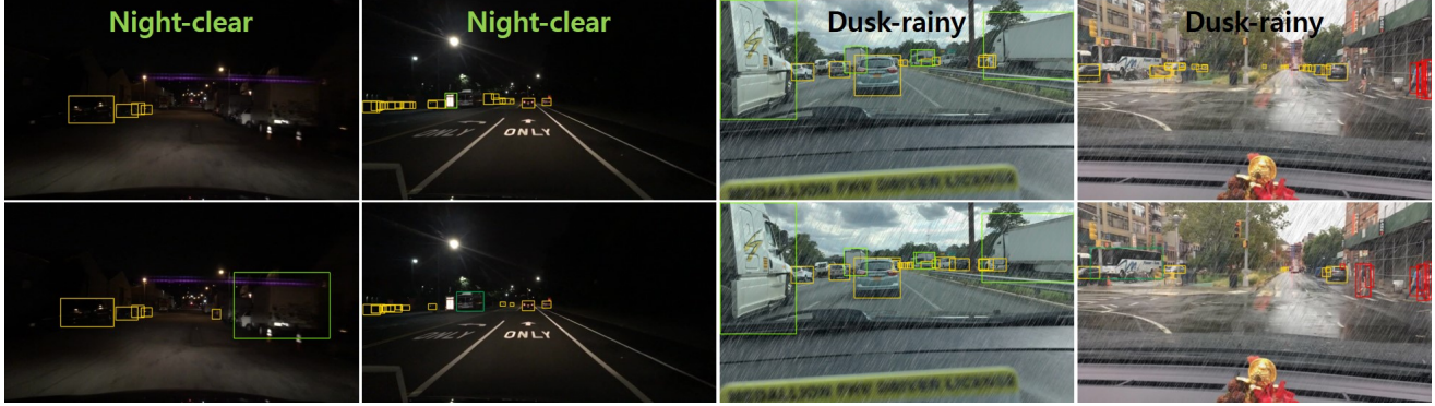
Figure 5. Qualitative Comparison. To evaluate performance on unseen domains, our model was trained using only daytime-sunny images. The top row shows results from the baseline detector, while the bottom row displays the results from proposed method on DWD [44].
