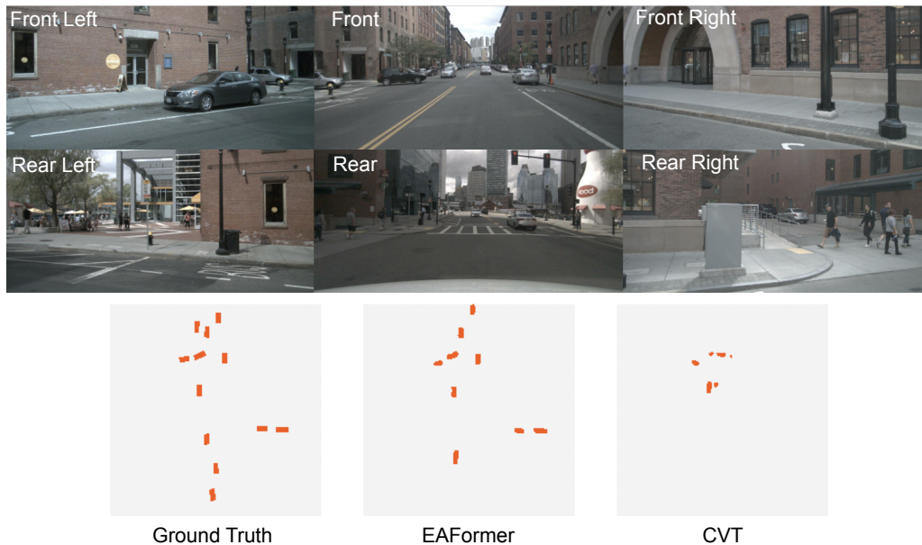
Figure 5. Visualization of zero-shot transfer performance of EAFormer and CVT for vehicle segmentation. The models were trained on Argoverse 2 (AV2) and evaluated on nuScenes.
