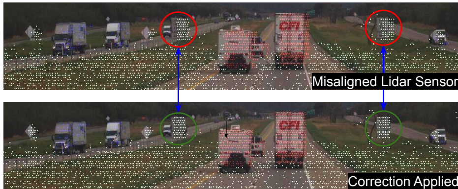
Figure 1. Demonstration of sensor misalignment correction using the proposed approach. The top image shows an input frame with visible misalignment when projecting the LiDAR data (green points) onto the camera image. In the bottom image, after applying the extrinsic parameter correction predicted by our model, the LiDAR points are well-aligned with the camera data, leading to improved 3D object detection accuracy.
