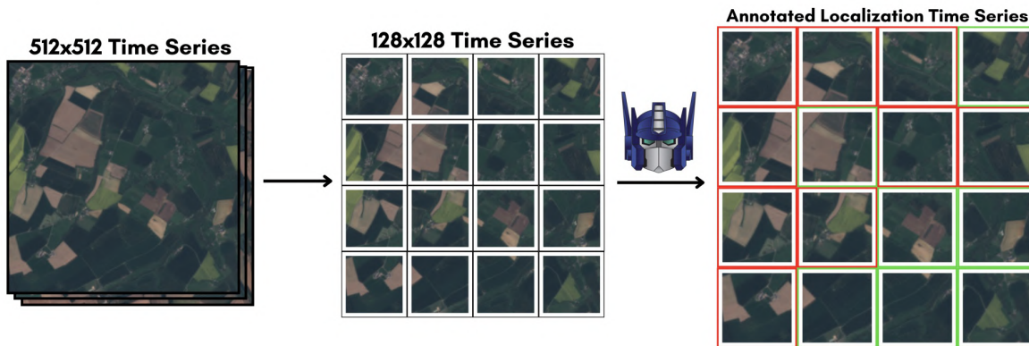
Figure 4. Illustration of the proposed pipeline for fine-grained change detection. Satellite image time series are divided into 128x128 patches to isolate localized changes, enabling the OPTIMUS model to classify each patch as exhibiting meaningful changes (e.g., urban expansion) or no significant change (e.g., seasonal variations). This approach addresses challenges in detecting changes across diverse components within larger images by focusing on spatially localized transformations.
