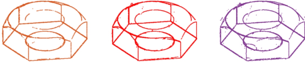
Figure 14. Comparison of 3D edge sketch results with different values of \Delta , for (Left) \Delta = 0.1 pixels, (Middle) \Delta = 0.3 pixels, and (Right) \Delta = 1.0 pixels, while \Delta\theta = 15^\circ and N = 4 views.
