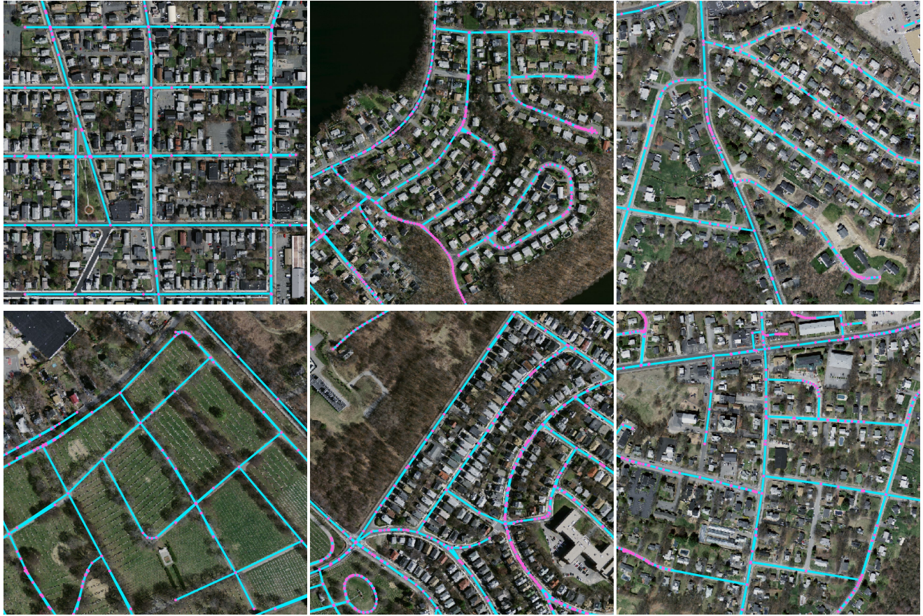
Figure 7. Qualitative results. Additional qualitative examples of road network predictions from the Massachusetts Roads dataset's test split.
