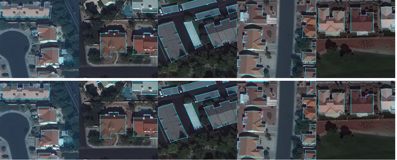
Figure 1. Qualitative comparisons. Examples of predicted building polygons from the INRIA test set. We compare between Pix2Poly (baseline) in the top row and Pix2Poly (ours) in the bottom row. The sequence prediction approach for vertex detection enables Pix2Poly to predict accurate and high-quality building polygons without the use of complex regularization losses, a differentiable rasterizer, and a topology feature learning module employed in competing methods. Zoom in for a better view.
