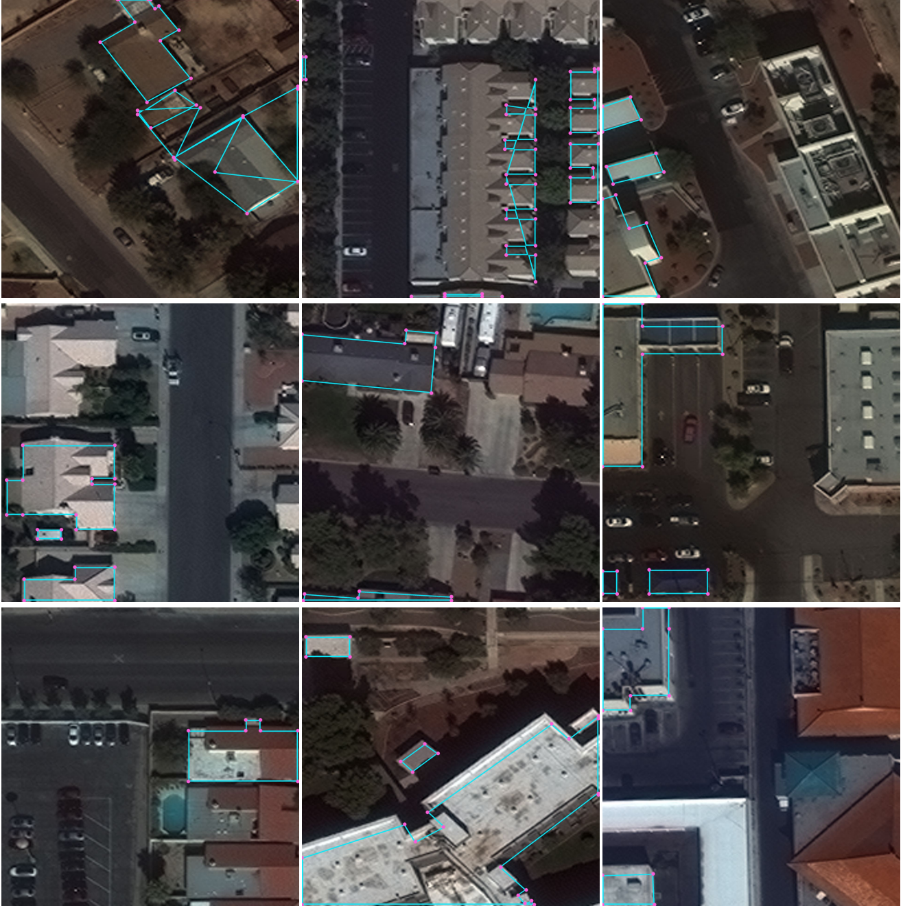
Figure 2. Failure Cases. Examples of some failure cases of Pix2Poly from the Spacenet Vegas dataset’s validation split. The most common causes of failure are partially or fully missing buildings in an image. Incorrect connections between vertices and overlap errors are also occasionally occurring failure cases.
