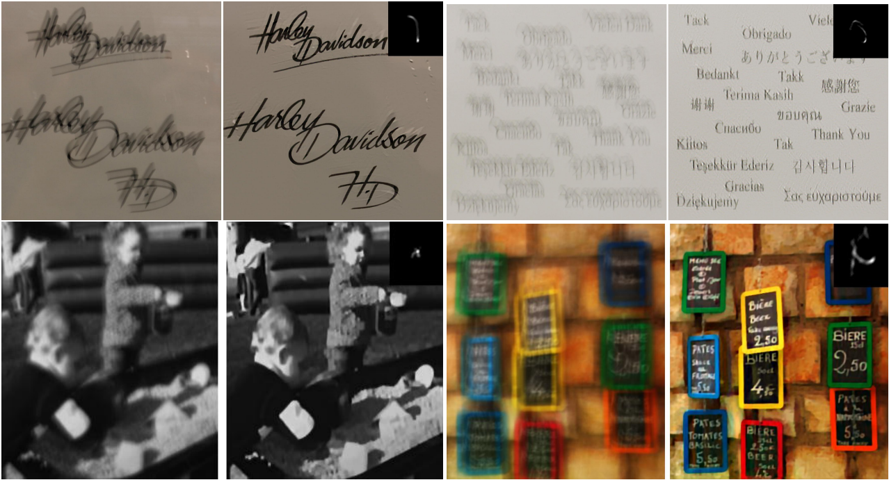
Figure 4. More results of our blind image deblurring algorithm, presented with the corresponding estimated blur kernel. For each pair, the input image is on the left, and the output of our algorithm is on the right for each pair.
