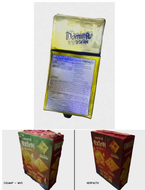
Figure 8. Examples of texturing artifacts generated with MVS-texturing [27]. Left: Illustration of MVS-Texturing mirage artifact. The text in the 03-sugar-box is distorted and repeated. We also observe color saturation on the blue separation line between the top of the box and the bottom. Right: Illustration of the MVS-Texturing color artifacts. The top of the 02-cracker-box on the left (COLMAP + MVS-Texturing) exhibit green areas that do not exist in the original model and are not produced by native texturing of other methods (e.g. Nerfacto on the right).
