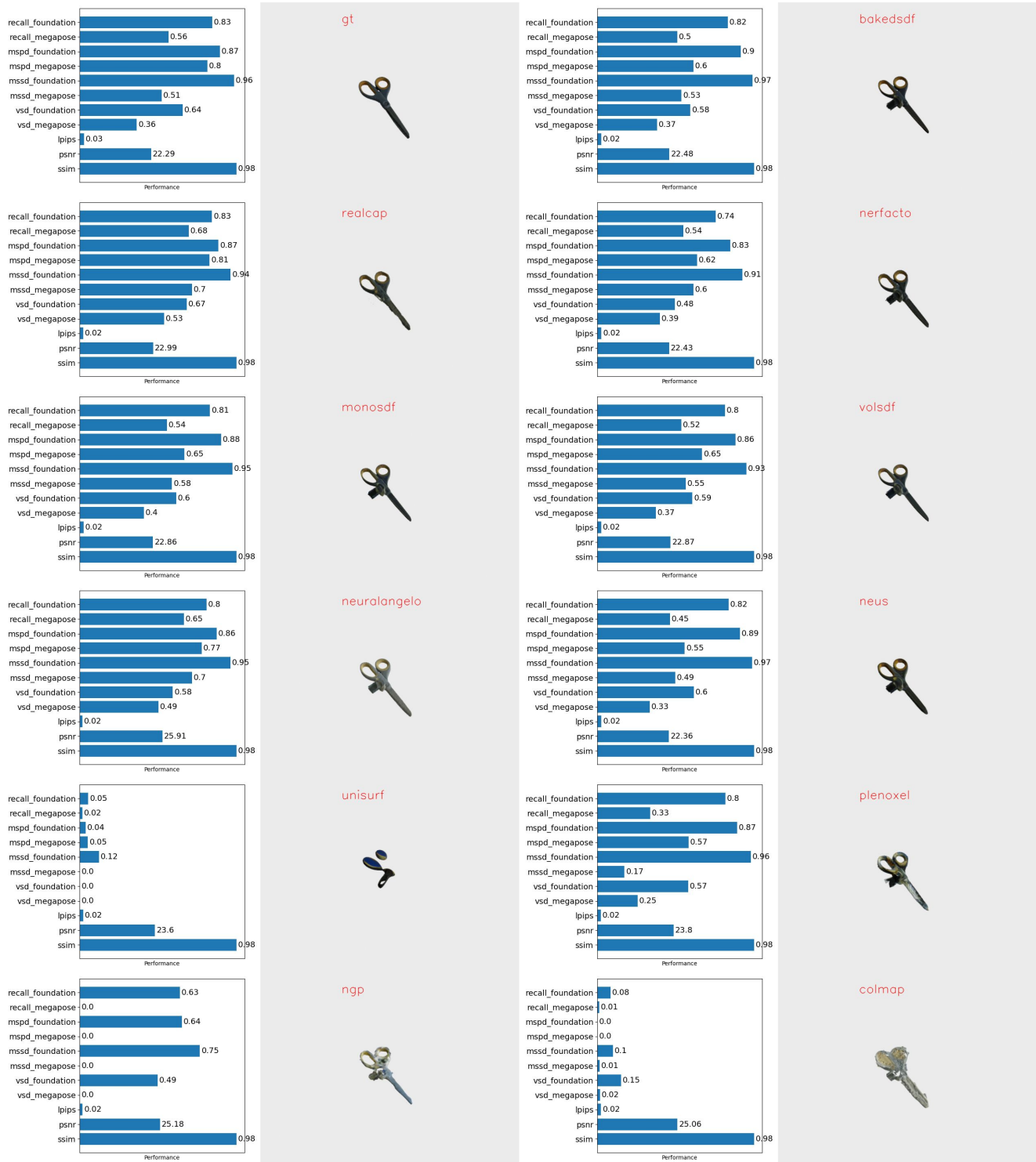
Figure 28. Pose performance and texture scores (left) and object renderings (right) of 17-scissors reconstructed with various reconstructed methods.
