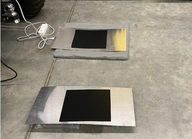
Figure 1. Approximate hot (top) and cold (bottom) uniform temperature sources used to compute the two-point NUC.
