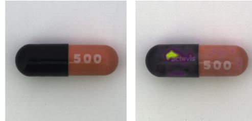
(b) Reference sample (left) and estimated anomaly map of ‘good’ test sample (right).
