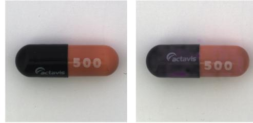
(a) Reference sample (left) and estimated anomaly map of ‘good’ test sample (right).
