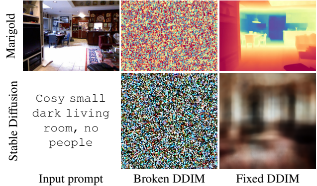
Figure A-1. Single-step outputs of Marigold and Stable Diffusion. With a single step, Stable Diffusion produces a blurry image at best, while Marigold outputs a sensible depth map. Note that the input prompt is text for Stable Diffusion, but an RGB image for Marigold.
