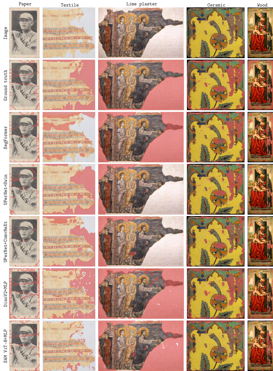
Fig. 3: Qualitative comparison for binary damage segmentation across Material categories.
