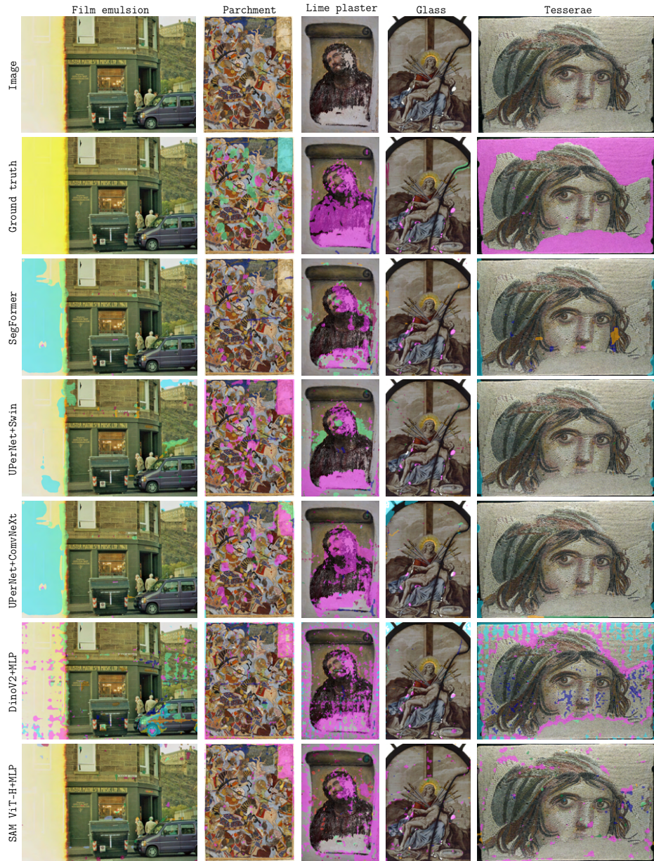
Fig. 5: Qualitative comparison for multiclass damage segmentation across Material categories.
