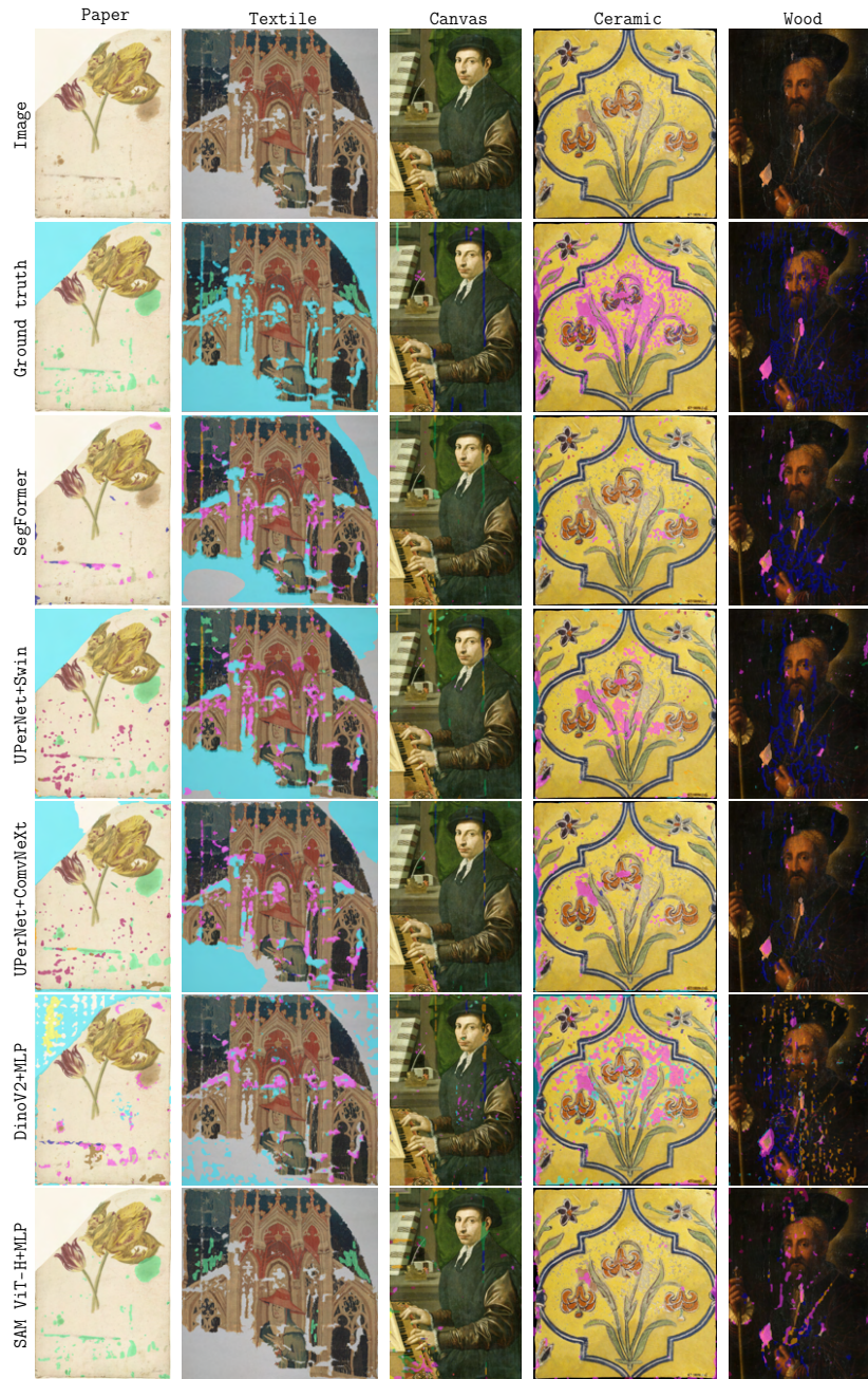
Fig. 5: Qualitative comparison for multiclass damage segmentation across Material categories.
