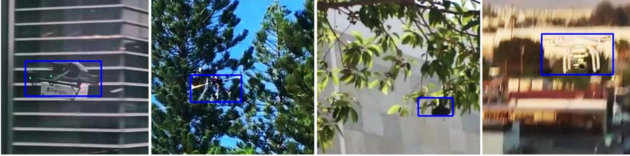
Figure V. Small cut-outs of selected samples from the DUT Anti-UAV test set that failed to be detected by YOLOv9e, irrespective of the employed training data. Ground truth bounding boxes are marked in blue.
