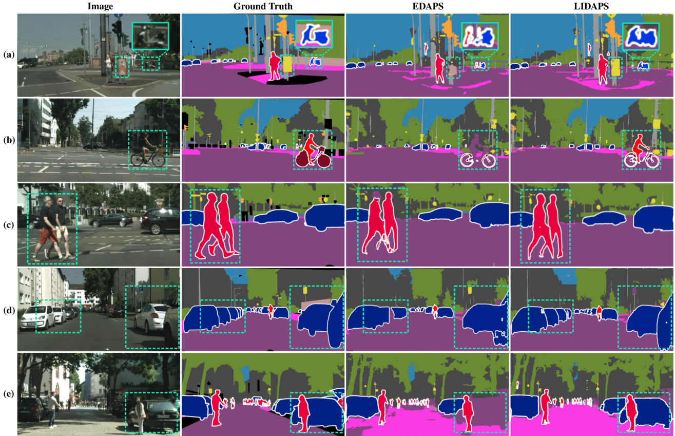
Figure 2. Additional qualitative results on SYNTHIA \rightarrow Cityscape UDA benchmark comparing EDAPS [10] to our proposed LIDAPS. Our proposed LIDAPS model predicts improved semantic and instance segmentation for several classes including “motor-bike” (a), “rider” (b), “person” (c) and “car” (d,e).
