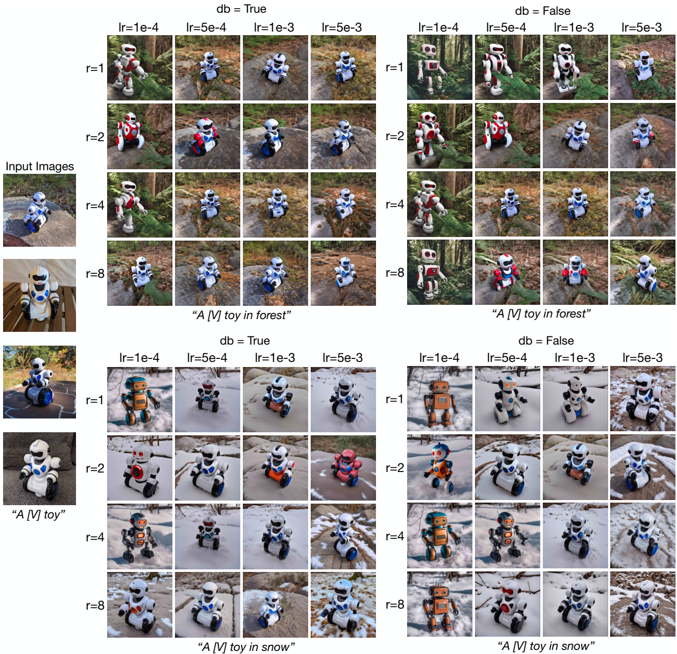
Figure 20. Ablation study on factor and learning rate for LoKr using SDXL, with a fixed factor of -1. We found that the optimal learning rate and rank are 1 \times 10^{-3} and 8, respectively. We also experimented with db=True , which indicates further low-rank decomposition of both matrices A and B , whereas db=False means only matrix B is decomposed further. (continued..)
