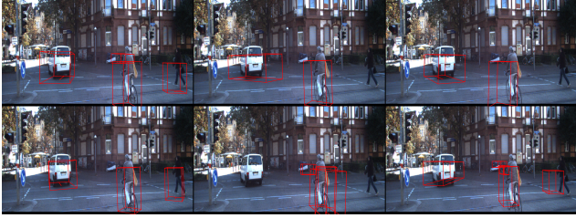
Figure 15. Predictions on KITTI. We test how the Particle-DETR trained on NuScenes generalizes to scenes in the KITTI dataset. Best viewed zoomed.
