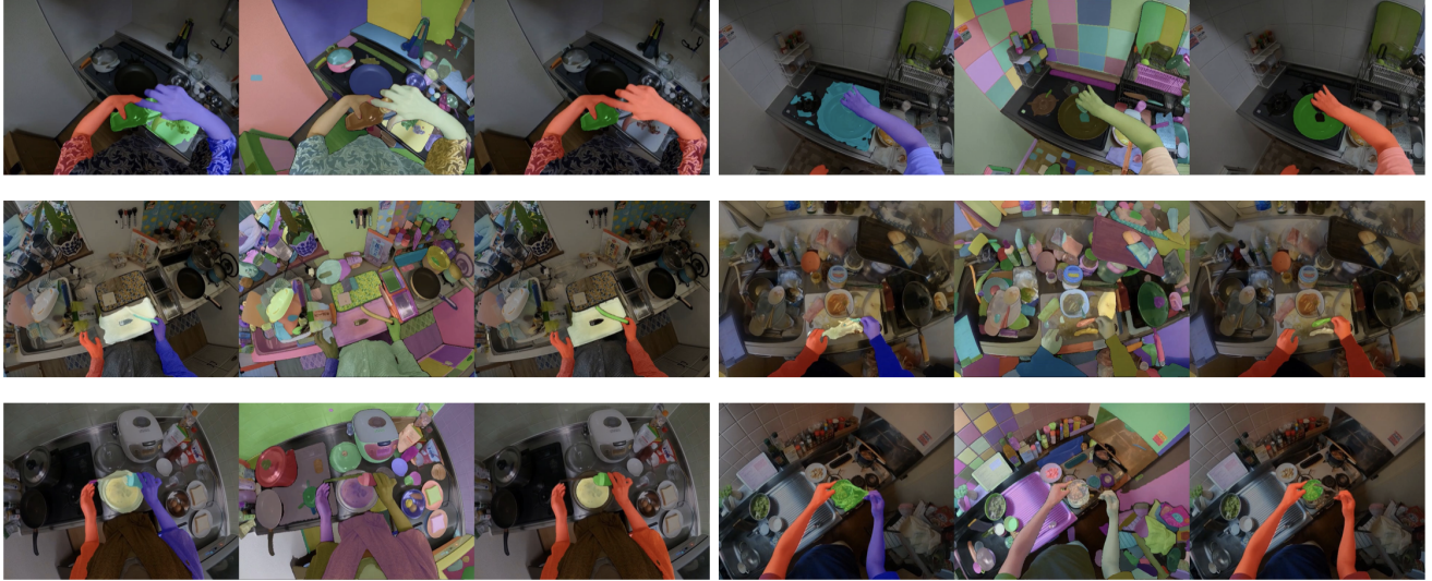
Figure 4. Our hand-object segmentation refinement. Each panel shows segmentation results of EgoHOS [11] (left), SAM [6] (middle), and our refined scheme (right), respectively. Since we don't use hand identity information (right/left), we show merged hand masks compared to the results of EgoHOS.
