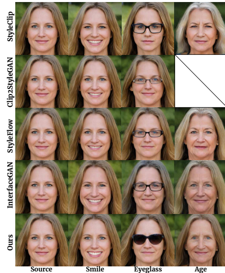
Figure 7. Qualitative comparison with single direction methods. StyleCLIP and CLIP2StyleGAN change the identity in age and eyeglass edits, respectively. InterFaceGAN entangles hair color with eyeglass attribute edits. StyleFlow changed the hair color while age editing. The proposed method can generate realistic edits without altering other attributes.
