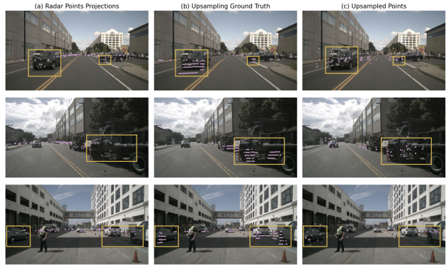
Figure 5. Visualization of upsampled points along with the original radar points and the sampled upsampling ground truth.
