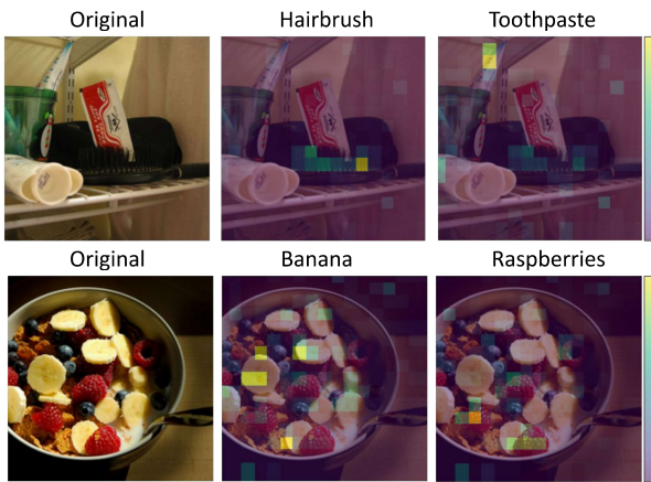
Figure 1. Additional results of token-level visualization. We overlay a sample image with attention maps between selected text tokens in generated response and vision tokens.
