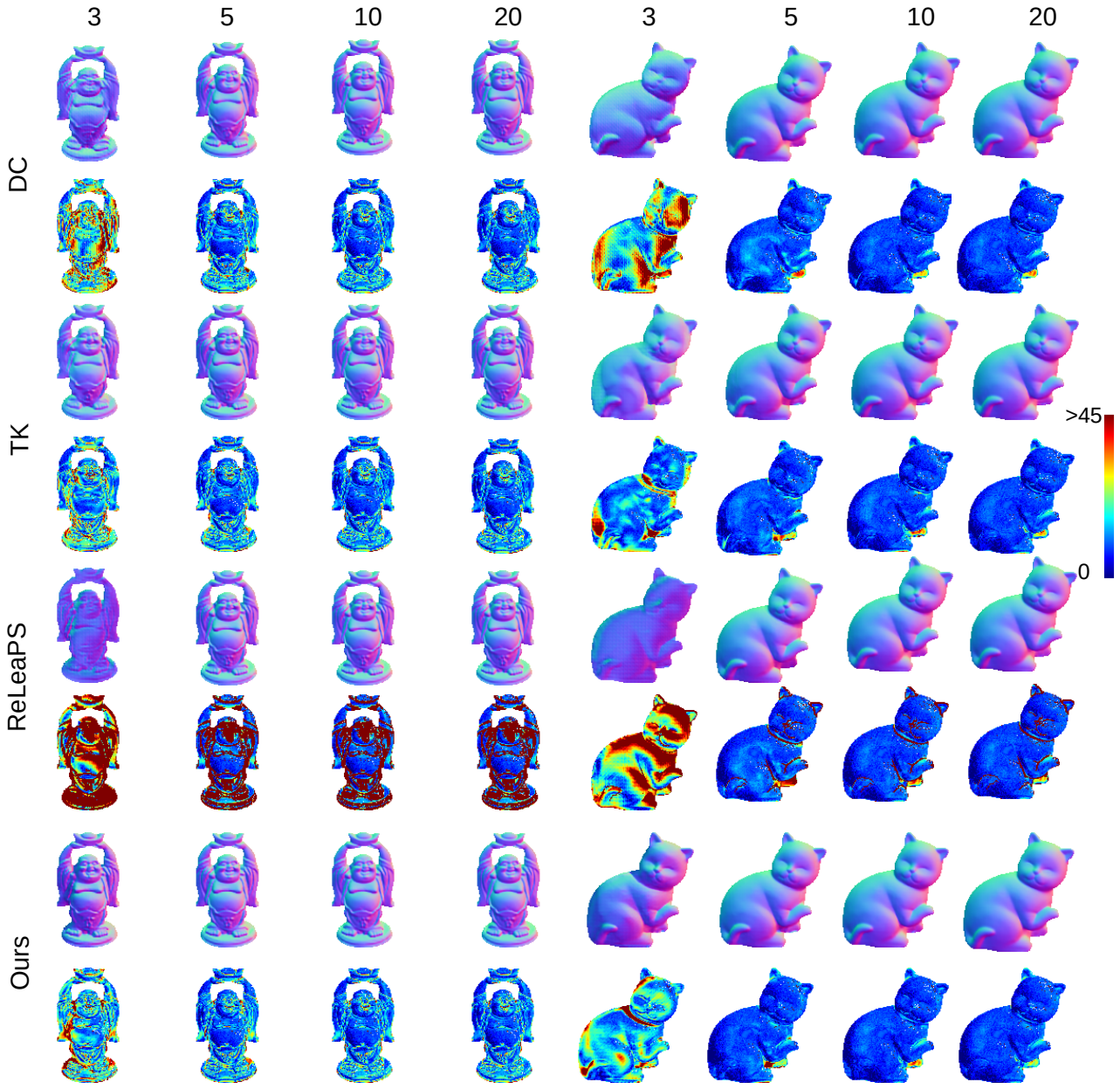
Figure 2. Qualitative comparison of variation of number of lights on the performance of different frameworks and different illumination planning methods over objects from the DiLiGenT dataset [3]
