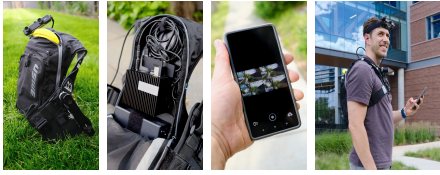
Figure 9. SANPO-Real Data Collection Rig.
