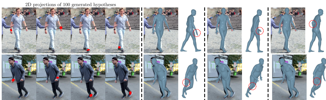
Figure S4. Examples demonstrating depth ambiguity for monocular 3D human mesh estimation. Although all hypotheses vary only slightly along the image directions, significant diversity for the depth is generated. Reprojections of 100 hypotheses for the right wrist, left wrist, right ankle, and left ankle are shown.
