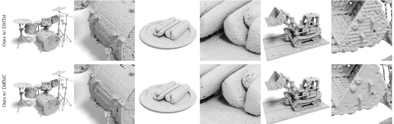
Figure 4. A mesh surface comparison of Ours between using DiffMC and DMTet reveals that DiffMC can create significantly smoother surfaces. This improvement is not limited to axis-aligned surfaces; it consistently outperforms DMTet on various rounded surfaces as well.
