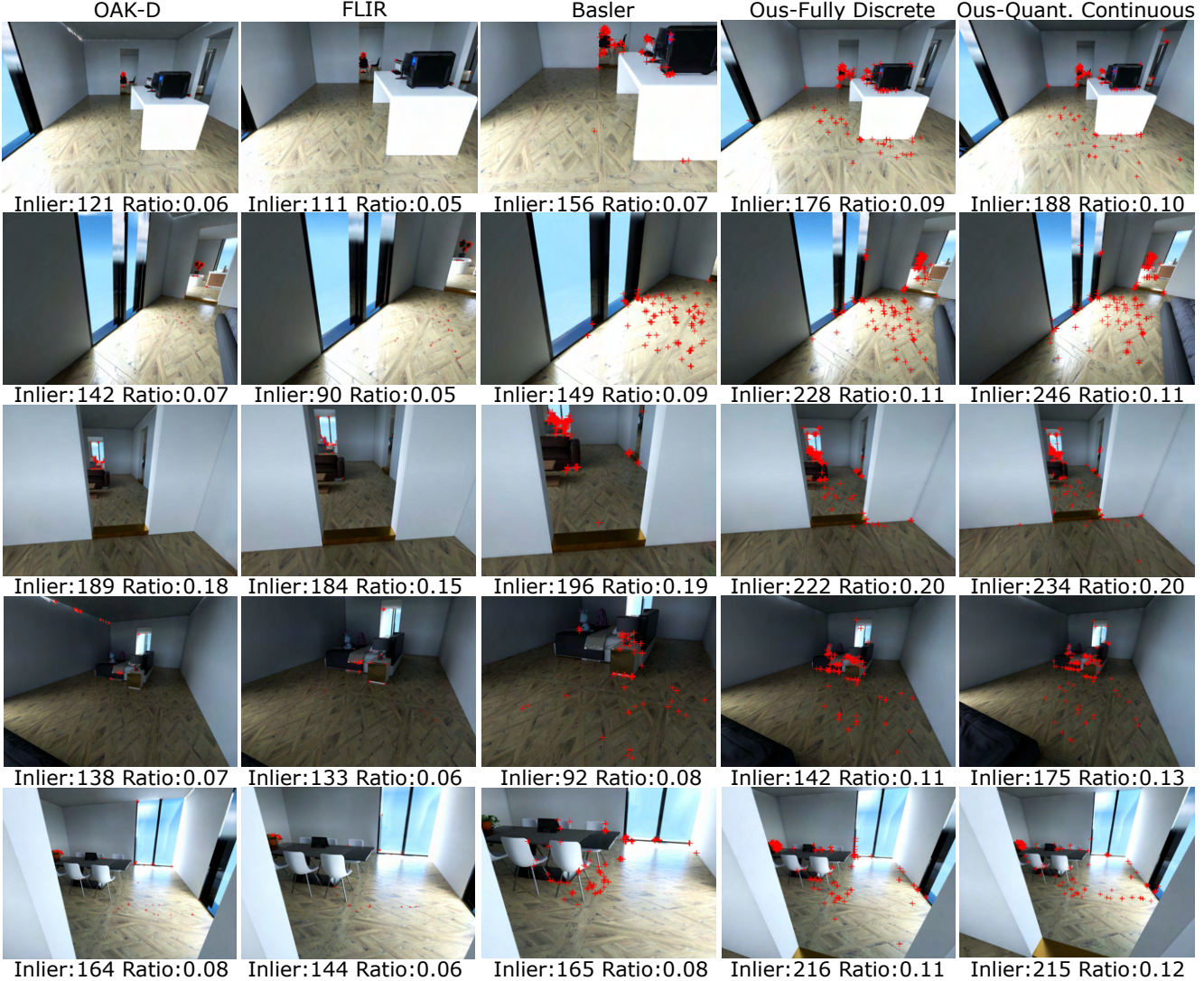
Figure 11. Comparison of feature extraction and matching with images captured by cameras designed by the proposed method and the off-the-shelf cameras. We display the features that are successfully matched with the features in the next frame and filtered (inliers) on the images, which shows that the cameras designed by our method contain the highest number of inliers.
