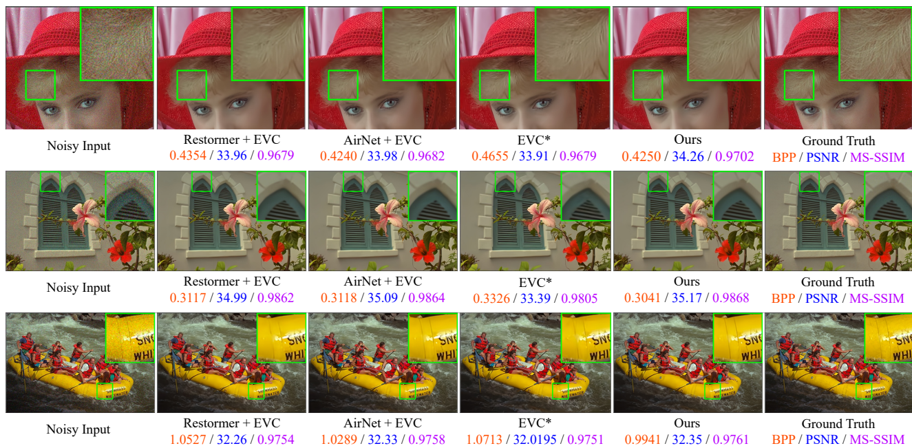
Figure 11. Qualitative comparisons on Gaussian noise-degraded images, where the noise level of input is set to \sigma = 15 . Results of cascaded solutions are denoted as restoration+compression . We report metrics of BPP/PSNR/MS-SSIM for each image.
