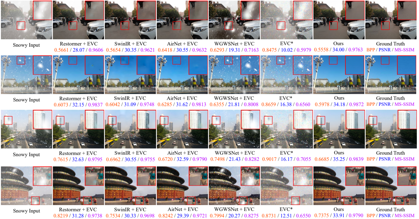
Figure 6. Qualitative comparisons on synthetic snowy images, where cascaded solutions are referred to as restoration + compression , and Ours denotes the results of Ours-L. For each image, we include metrics of BPP/PSNR/MS-SSIM .
