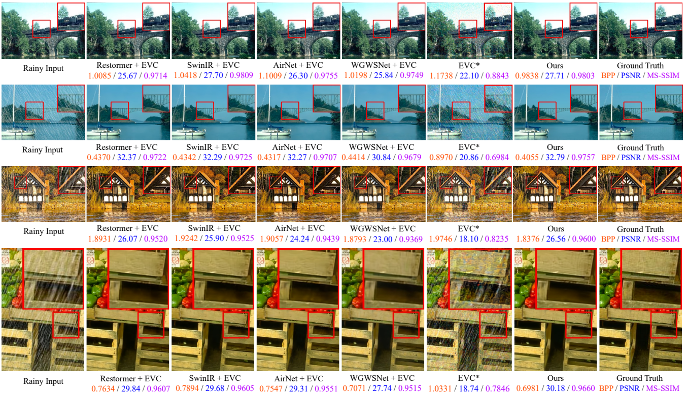
Figure 7. Qualitative comparisons on synthetic rainy images, where cascaded solutions are referred to as restoration + compression , and Ours denotes the results of Ours-L. For each image, we include metrics of BPP/PSNR/MS-SSIM .
