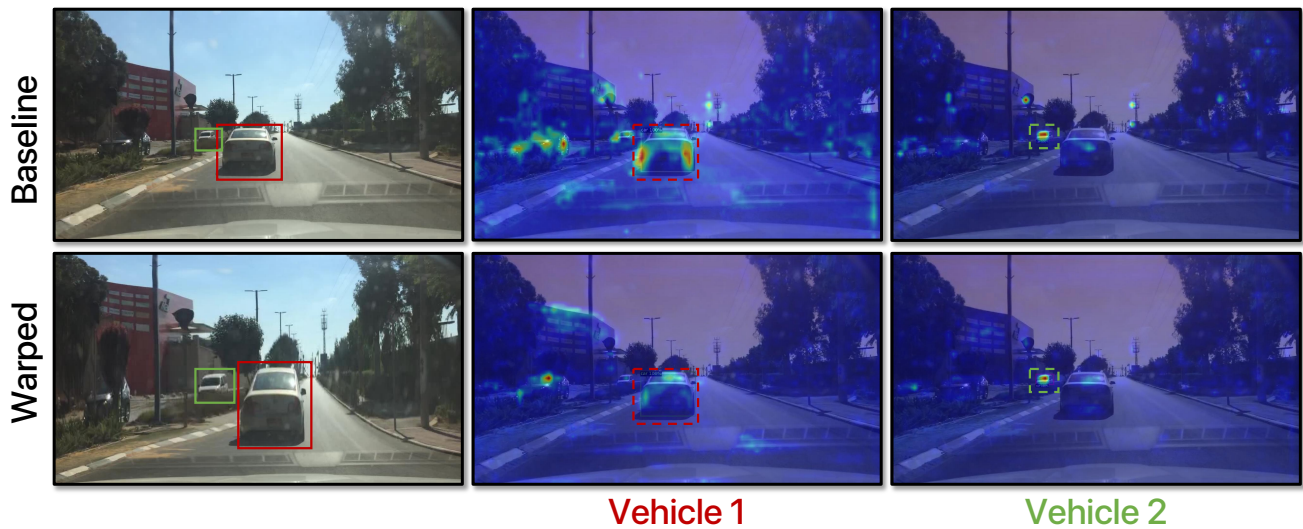
Figure 4. Additional Analysis: Grad-CAM [14] Visualizations for Multiple Objects. We observe that learnt features show smaller Gradcam visualization contributions from background pixels compared to foreground object pixels when trained with instance-level warping. This is true for individual object instances, in this case, for Vehicle 1 and Vehicle 2. This suggests that our instance-level warping enhances the model’s focus on foreground object pixels over background pixels.
