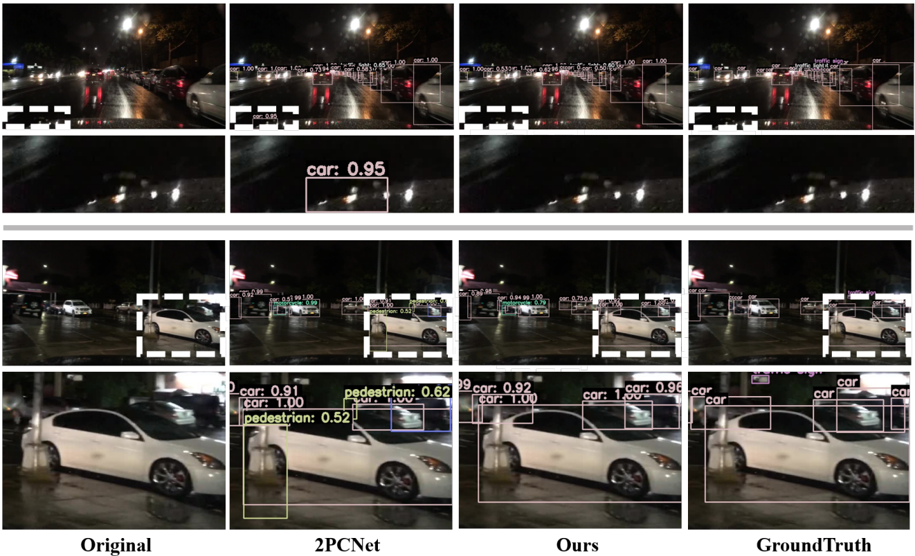
Figure 7. Additional Analysis: BDD100K (Clear → Rainy) Object Detection. Our method demonstrates superior object detection under rainy conditions by accurately identifying vehicles and minimizing false positives, such as misidentified pedestrians and cars evident in 2PCNet [8] predictions.
