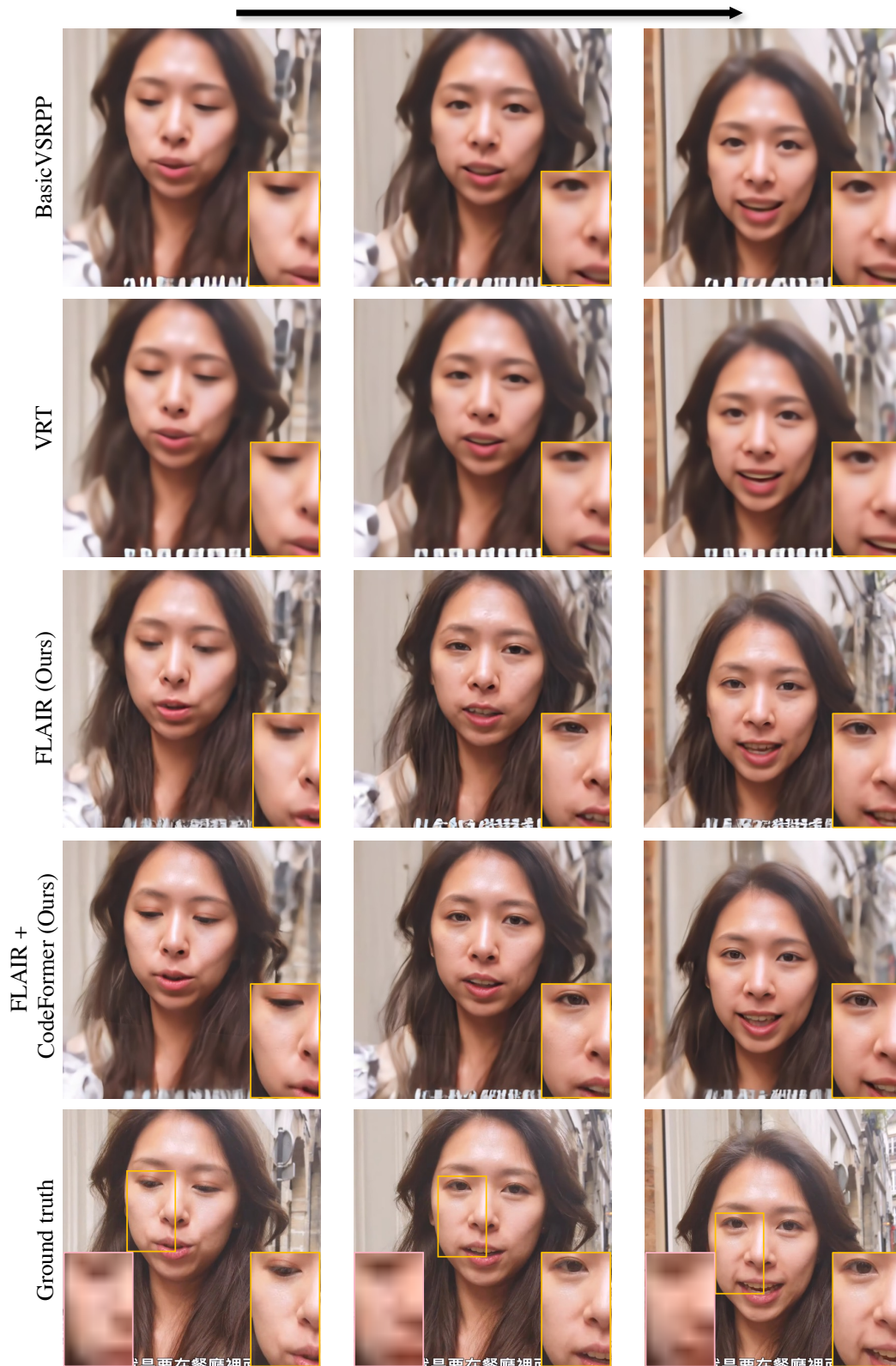
Figure 13. More visual comparisons of 16\times face video super-resolution on CelebV-Text [25]. Each row consists of three video frames, with an interval of five frames between each selected frame. The zoomed-in regions of each method are displayed in yellow boxes, along with their LQ counterparts in pink boxes. Best viewed by zooming in the display.
