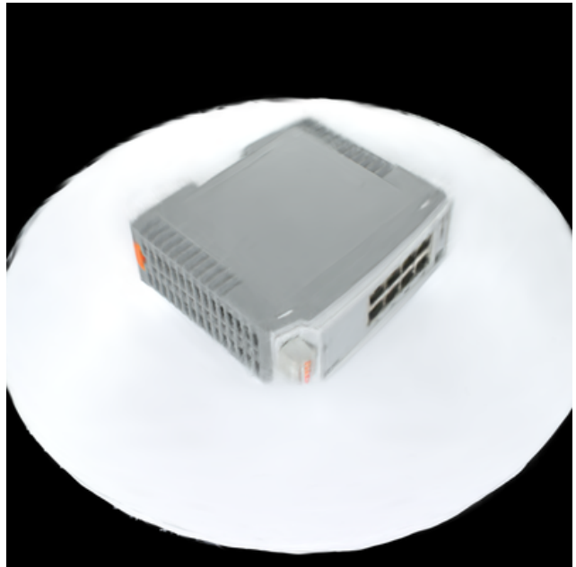
Figure 11. Example for result from 3D gaussian splatting for product Switch (8 x RJ-45) .
