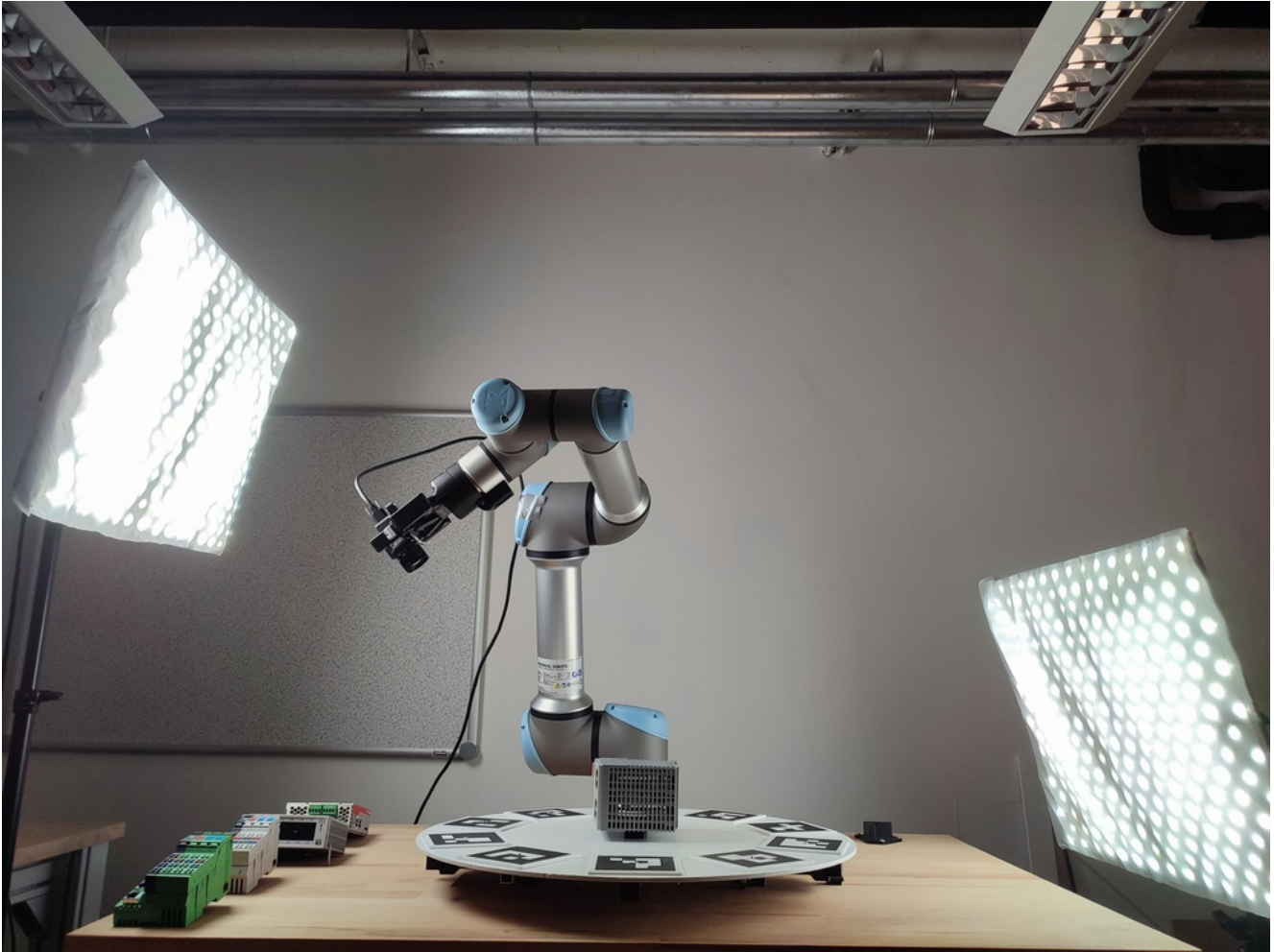
Figure 6. Hardware setup for the dataset acquisition from the side. The servo motor is fixed to the table from the bottom-side and the axis is attached to the circular plate. The light panels to the left and right are fixed in position for the acquisition of the main dataset. For the secondary dataset with variations in lighting, the light panels are randomly shifted to induce shadow casting. The camera is attached to the tip of robot arm. The gripper of the robot arm is not utilized and kept open.
