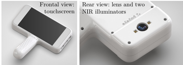
Figure 1. Frontal and rear views of the handheld newborn iris scanner custom-designed for this study by an industrial partner.
