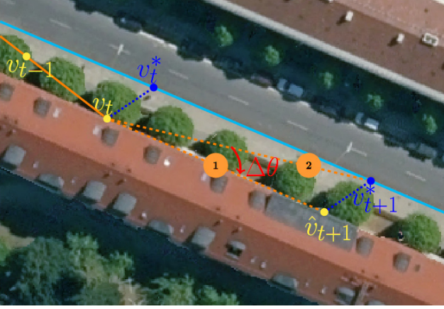
Figure 2. Visual representation of how Slope Penalty loss can be calculated. The ground truths are denoted by cyan lines and predicted edges by orange lines. Yellow nodes represent predicted vertices and blue nodes represent their corresponding ground truth label.
