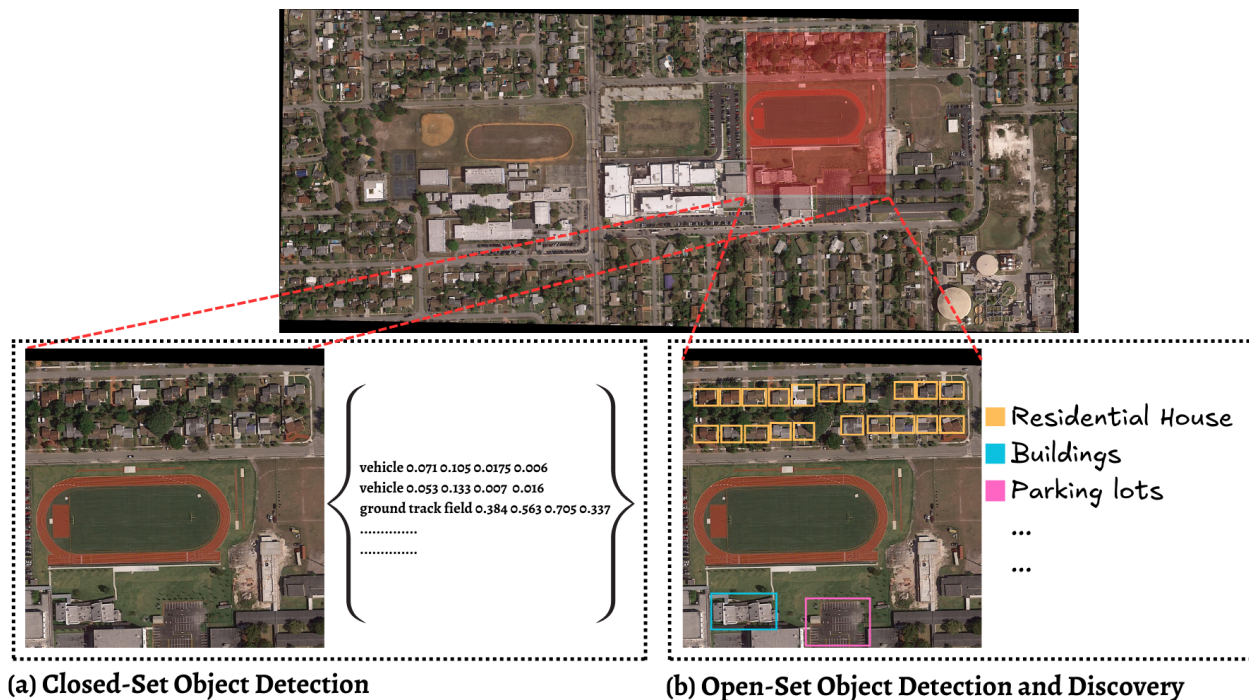
Figure 1. A visual comparison of the object detection task in closed-set and open-set scenarios. In closed-set object detection, the detection model is trained using known class label information and ignores any novel classes. In contrast, open-set object detection and discovery aim to identify and categorize both known and unknown classes within an image, enhancing scene understanding and the learning paradigm.
