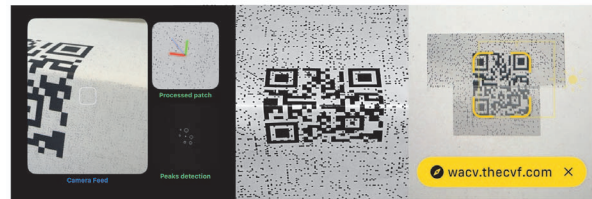
Figure 1. A self-rectifying texture and a QR code are printed on a piece of paper folded across a table edge. This deformation prevents the QR code from being read. By contrast, the real-time self-rectifying texture reader (left) can acquire the deformation differential (left lower inset) from the small patch being processed (left upper inset); from this single patch, after affine rectification, the traceability information is easily decoded. A photograph of the QR code spread across two surface faces (center) cannot be read. However, the geometric information exposed by the self-rectifying texture easily allows rectification of a homography for each planar surface, allowing the QR code to be read.
