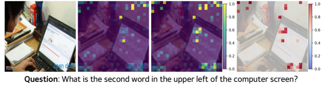
Figure 5. Visualization of the effect of Cross-resolution Token Scoring. The left shows the intra-resolution token scores, the middle presents the final scores obtained by combining intra- and cross-resolution token scores, and the right highlights the difference between the final and intra-resolution scores.
