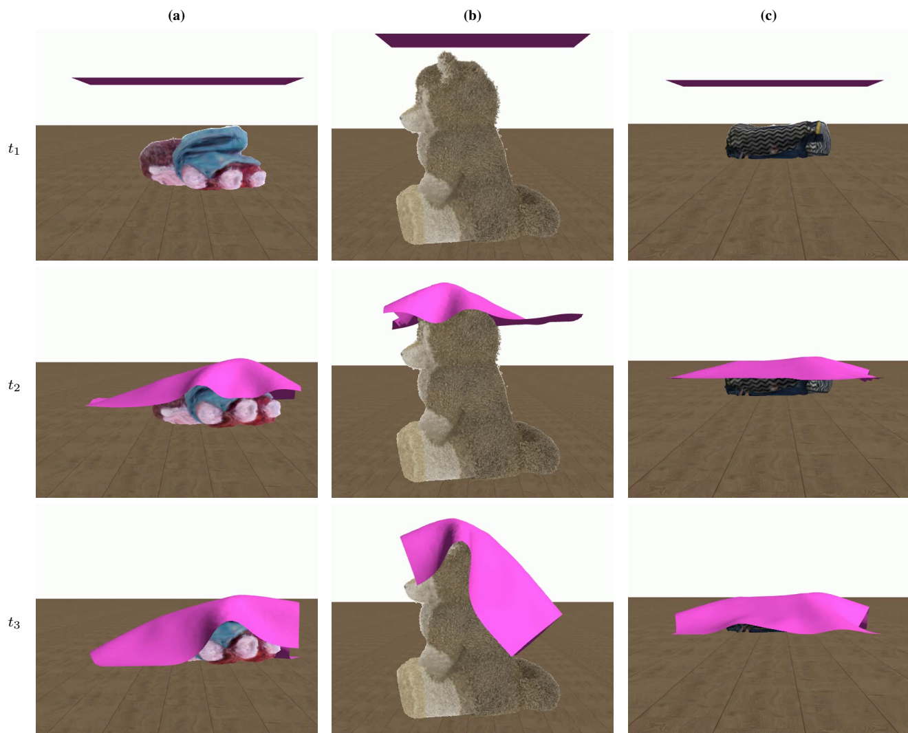
Figure 5. Sampled frames from the cloth PDB solver and 3DGS interaction at three timesteps ( t_1 – t_3 ). Columns (a)–(c) show three 3DGS models for each instant.
