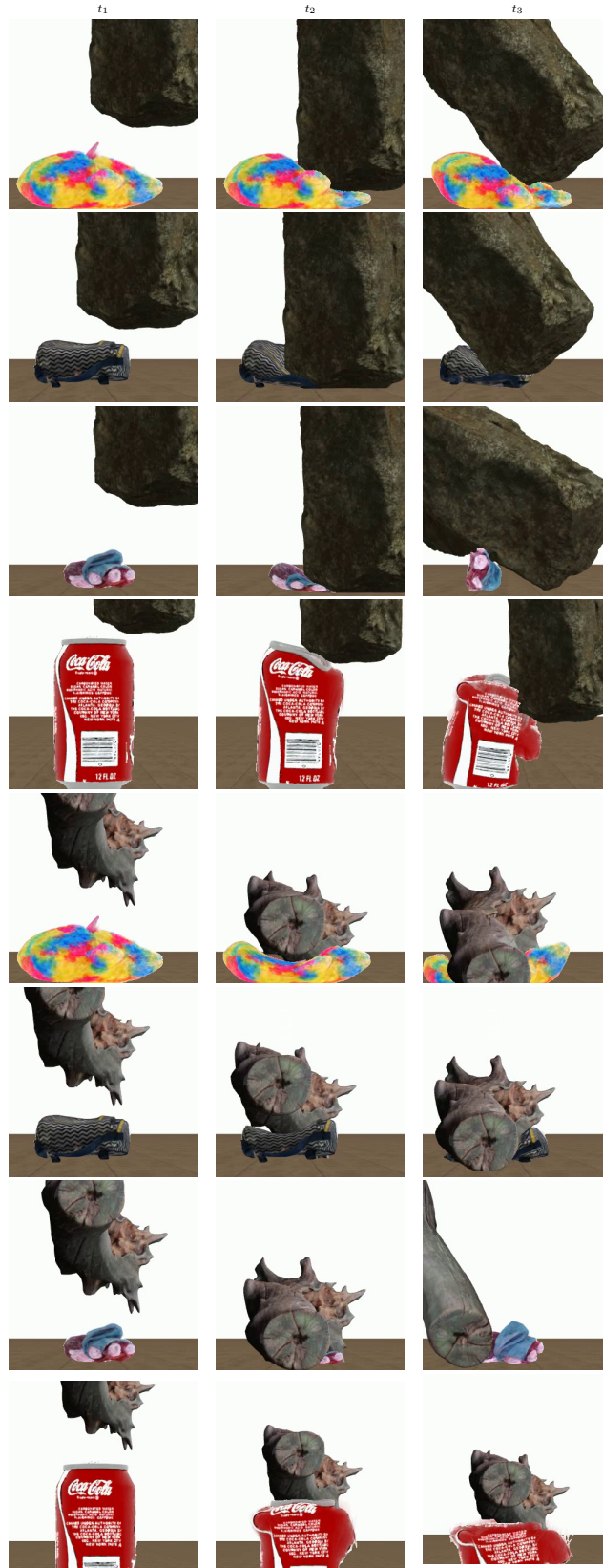
Figure 4. Temporal comparison of mesh-3DGS interactions (transposed layout). Columns correspond to timesteps ( t_1 - t_3 ). Rows correspond to distinct interaction scenarios (rock or log impacting different 3DGS objects). It can be seen that this interaction results in physically plausible simulations.
