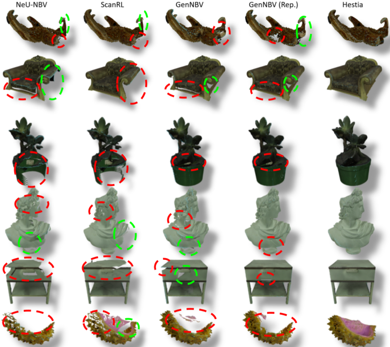
Figure S2. Qualitative comparison on OmniObject3D [23]. Hestia’s viewpoints reconstruct the point clouds of real-world scanned objects accurately, while other baselines exhibit less robustness across various object shapes, often missing parts in the reconstructed point clouds.
