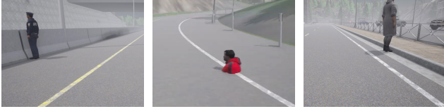
Figure 3. Examples from the ARCAN project (CARLA-BSP): scenes featuring a single pedestrian in crossing/non-crossing situations, following binary or simplified behavior labels.
