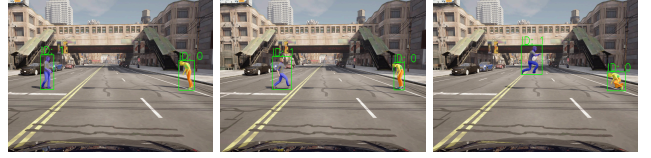
Figure 8. Multi-frame detection, segmentation, and tracking. Consistent track IDs, even in edge-case motions, highlight pose consistency and temporal coherence of HABIT.
