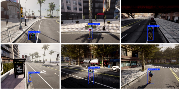
Figure 7. Zero-shot pose estimation on simulated data. Qualitative results of YOLOv11-pose applied to HABIT.
