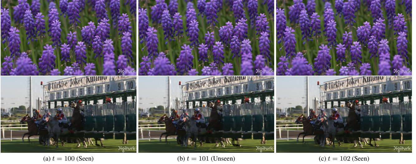
Figure 7. Frame interpolation. For low-motion videos (top), GaRV has strong interpolation capabilities. For high-motion (bottom), GaRV may distort object edges – see the letters/numbers.
