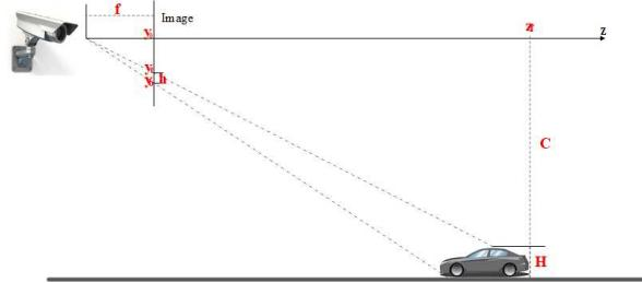
Figure 3. The perspective geometry between vehicles and camera.
