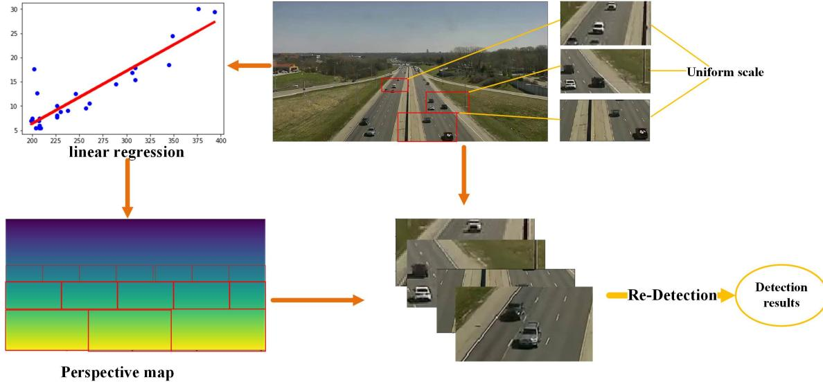
Figure 4. Firstly, according to the initial detection result, the perspective map is solved with linear regression map, and then the area is cropped to ensure that the capacity of each region is consistent. The final detection result is obtained through re-detection. As shown in the upper right corner, after the divided area has been resized, the vehicle maintains a consistent size.
