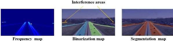
Figure 2. From left to right, it respectively represents the effect of binarization and filtering small connected areas. As shown in the middle figure, the small connected regions are often interference areas such as parking lots or houses.
