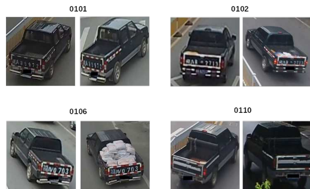
Figure 1. Examples of similar vehicles with their identity numbers in VeRi-776 dataset [20]. These pickup trucks have almost identical model and color, which makes vehicle Re-ID extremely challenging. One possible solution is to extract more discriminative local features from distinct regions.
