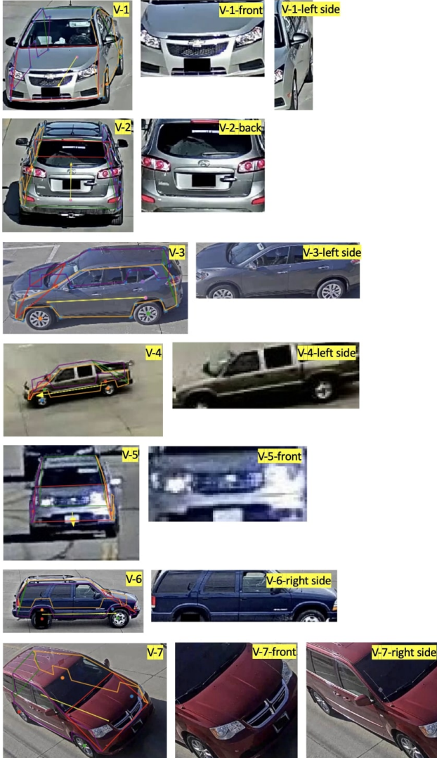
Figure 7. Examples of vehicle keypoints detection and visibility estimation. keypoints are marked in blue dots, occlusion parts are estimated. The red, green, orange and purple outlines indicate the front, back, left side and right side, respectively. The yellow arrow represents the driving direction \vec{r} . Cropped views of visible surfaces are shown as well.
