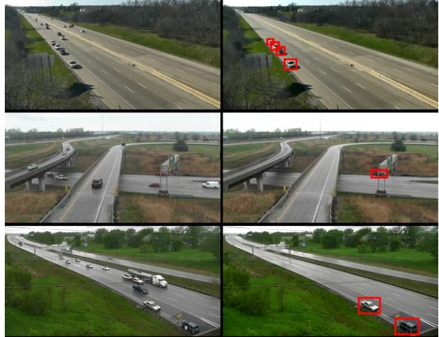
Figure 5. Examples of detected anomalies on the Iowa DOT Traffic Dataset. Original video frames are shown on the left, and processed video frames with detected anomalies from [39] are shown on the right.
