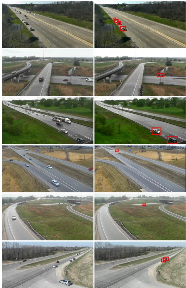
Figure 9. Examples of detected anomalies. Left column: the original video frames. Right column: the corresponding processed video frames with detected anomalies shown with red bounding boxes from background regions. Other vehicles are smoothed out using our proposed method.
