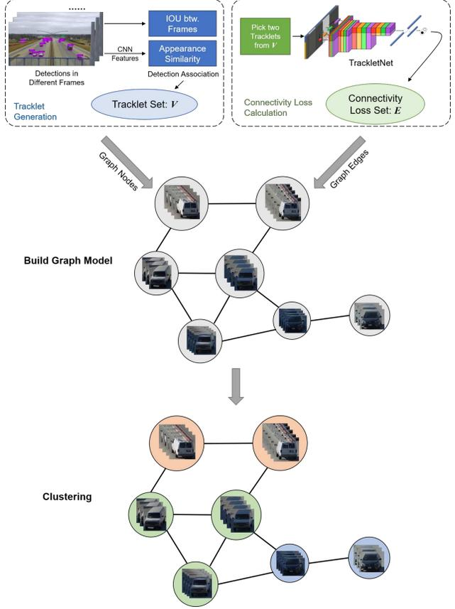
Figure 5. The TNT framework for multi-object tracking. Given the detections in different frames, detection association is computed to generate Tracklets for the Vertex Set  $V$ . After that, each pair of two tracklets are put into the TrackletNet to measure the connectivity, which formed the similarity on the Edge Set  $E$ . A graph model  $G$  can be derived from  $V$  and  $E$ . Finally, the tracklets with the same ID are grouped into one cluster using the graph partition approach.
