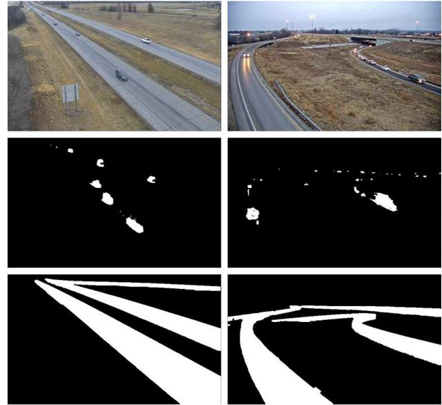
Figure 2. Examples of background modeling and traffic flow mask. From the top row to the bottom row: original video frames, foreground masks after background subtraction, traffic flow masks, respectively.
