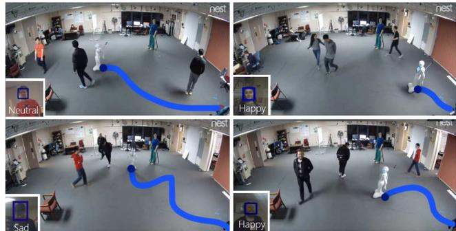
**Figure 1:** We present a real-time data-driven planning algorithm that learns about pedestrians' emotional state in order to navigate socially aware. The robot learns in real time about the emotions of pedestrians and their proxemic constraints. These distances limit the movement and navigation of the robot to avoid intrusion into peripersonal and interpersonal social spaces of the pedestrian. Combining emotional and proxemic constraints enhances social comfort as well as navigation.
