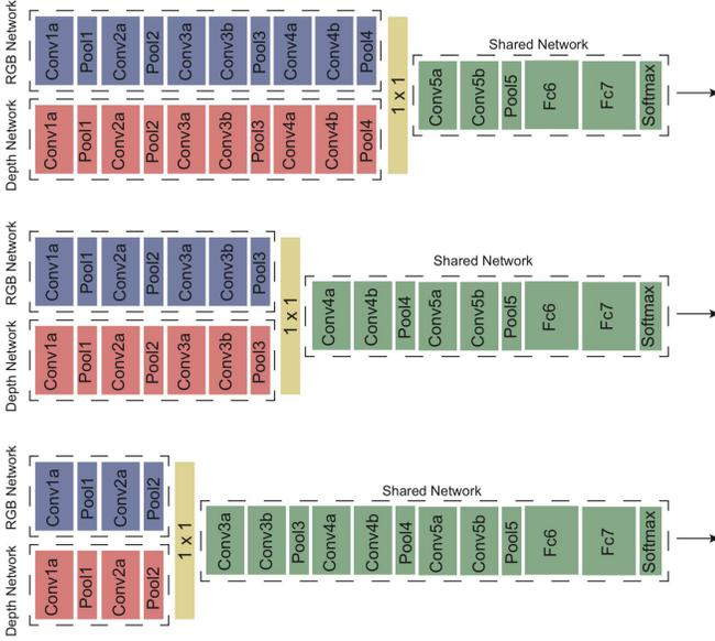
Figure 3: Overview of the proposed intermediate fusion module via  $1 \times 1 \times 1$  convolutions. We combine the two streams at different levels of the network *i.e.* at the second, third and fourth pooling layer. After the fusion module the two streams are merged to a single shared network using concatenation.
